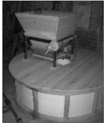
Fancroft-New millstone enclosure and hopper.
